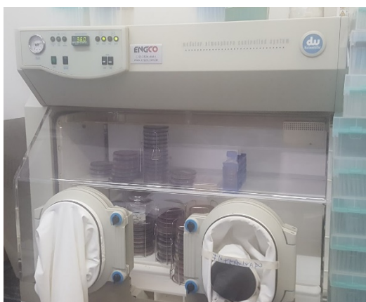
Figura 13 - câmara de anaerobiose MiniMacs Anaerobic Workstation (Don Whitley Scientific, Bingley, West Yorkshire, UK)
